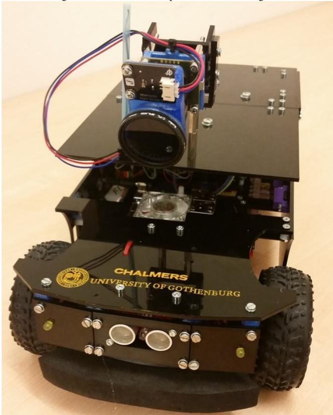
contour. The camera is positioned in a such a way that the left line is only visible in, assuming we cut the frame in 4 equal sectors, the top left sector of the image.
