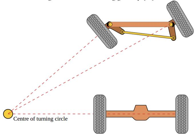
Only cars based on Ackermann steering, or variations of, are allowed to compete [Fig. 6]. Ackermann steering is the standard for commonly met automobiles.
