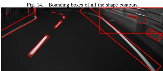
Fig. 14. Bounding boxes of all the shape contours.
